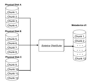
The total capacity of this concatenated metadevice is the combined capacities of the three drives. If each drive is 4 gigabytes, for example, the metadevice has an overall capacity of 12 gigabytes.
